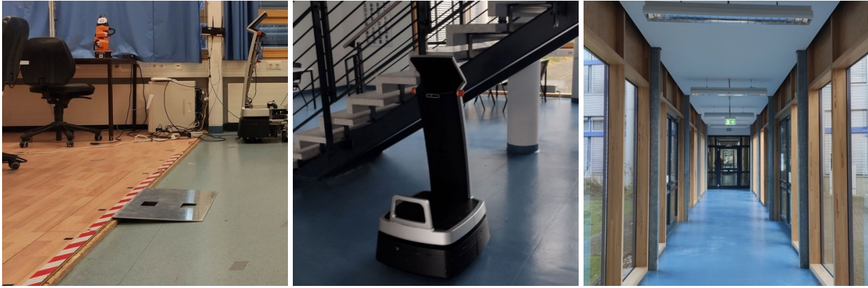
Figure 1: Challenging architectural elements for occupancy grid maps: (a) small floor elevations, (b) low hanging structures, and (c) walls predominantly made of glass panels
