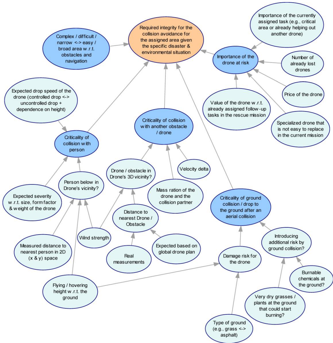
Figure 20 Conceptual SINADRA model (b) for the risk variability w.r.t. the required integrity for the collision avoidance given the situation & environment.
